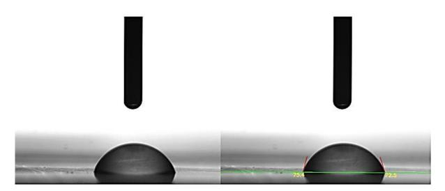
Sample images of contact angle measurement. The image on the left is the raw image, and the image on the right has been analyzed using Jikan Assistant software.
