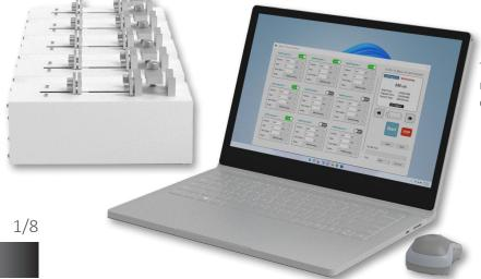
The Jikan SPM-Lite supports simultaneous control of up to eight devices via the Jikan software.
