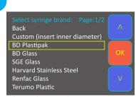
After selecting the syringe type in the first page, the syringe volume should be selected from the available list of values. The user can also enter a custom diameter in case the desired volume cannot be found in the database.
